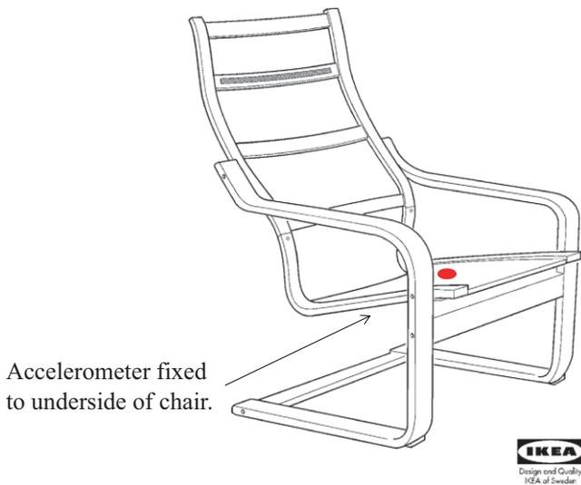
**Figure 1.** Drawing of a Poang (Ikea, Inc.) model chair (minus cushions) indicating the location of the accelerometer.
