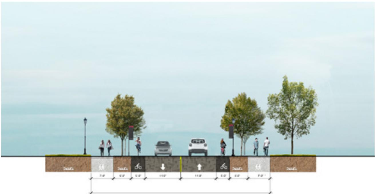
FIGURE 36: ASBURY AVENUE—PROPOSED STREET SECTION, LOOKING EAST
