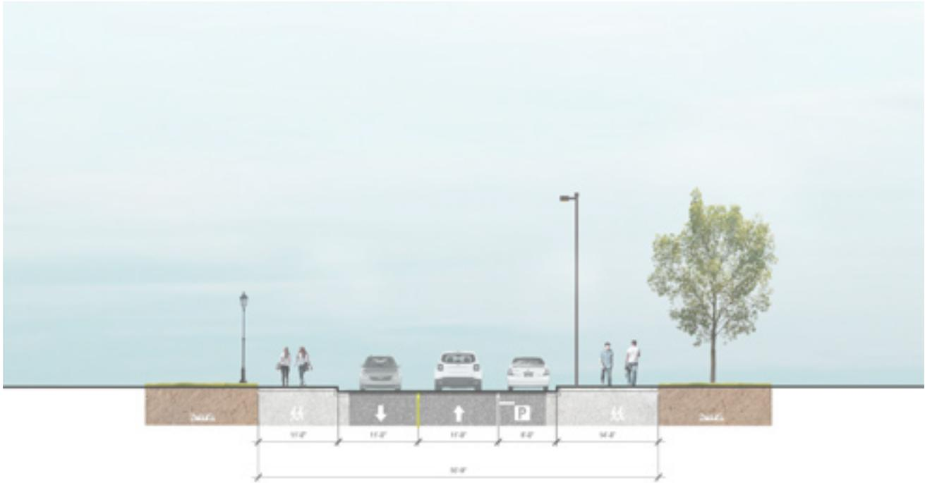
FIGURE 35: ASBURY AVENUE—EXISTING STREET SECTION, LOOKING EAST
